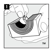
Adapt modules, which are to hold cables or pipes, by peeling off layers until you reach the gap seen in pic. 2. The halves may not differ by more than one layer.
